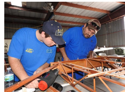
Figure 31 (Image credit: EAA and General Aviation News) Student member being taught how to assemble wing rib.
